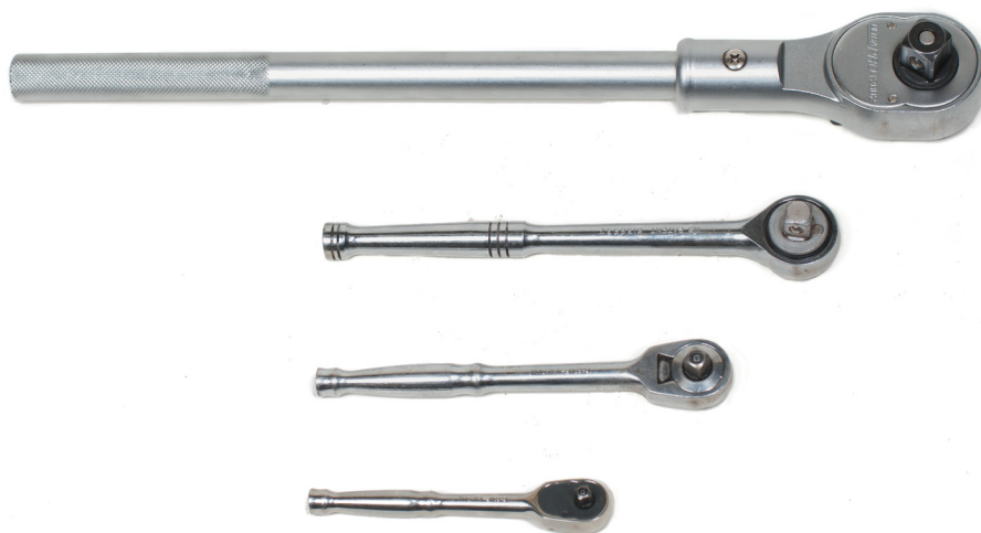
Figure 43 —Ratchets with different-sized drives: 1/4", 3/8", 1/2", 3/16"
